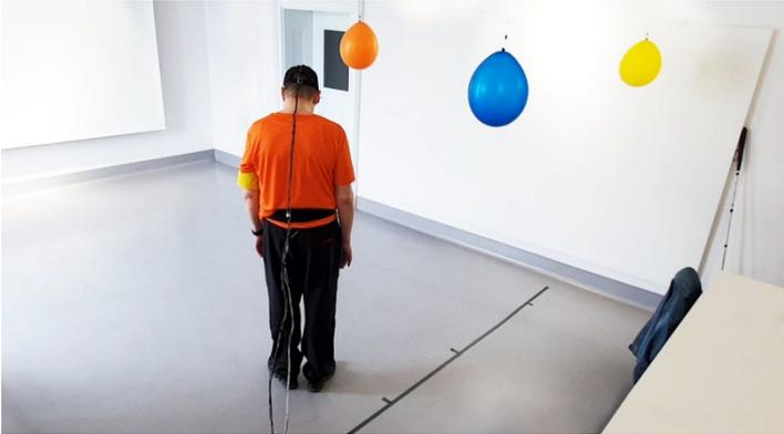
Figure 11-3: Anti-collision experiment with three balloon obstacles. The participant wears the prototype consisting of a camera cap and textile belt with three integrated Peltier modules to provide left, stop, and right commands. [12] p 171
